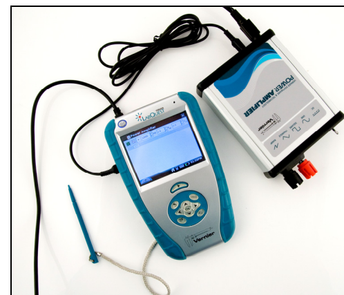
Power Amplifier connected to a LabQuest and a computer
