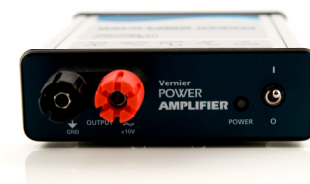
The front of the Power Amplifier, showing the output terminals, the Power Indicator LED, and the On/Off Switch
