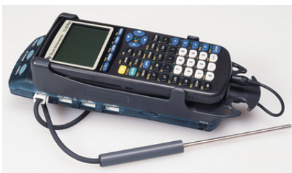
LabPro interface, TI-83 Plus calculator, and Stainless Steel Temperature Probe
