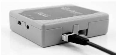
A digital sensor attached to LabQuest Mini
