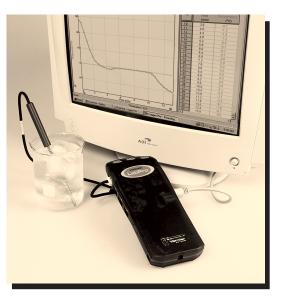
To make LabPro easier to use, we added many new features, the most important being automatic sensor recognition. When you plug in a new auto-ID probe, LabPro loads the calibration and other
