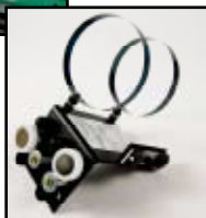
Hoop spring used to launch cart
