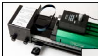
Hoop spring used to launch cart
