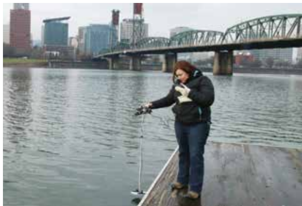
Colleen McDaniel lowers the PAR Sensor and Secchi disk into the Willamette River
