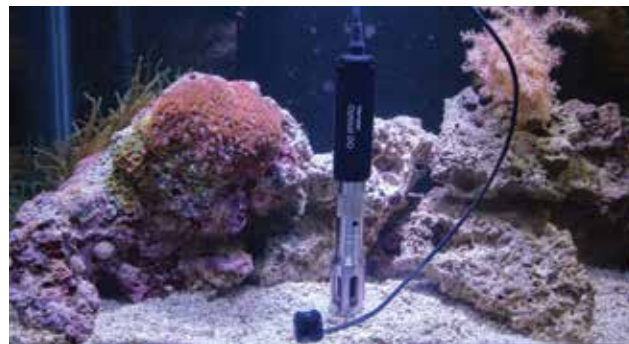
Measuring photosynthetic light levels and dissolved oxygen concentration in the saltwater aquarium using the PAR Sensor and the Optical DO Probe
