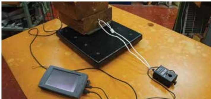
Setup for coefficient of kinetic friction demonstration
