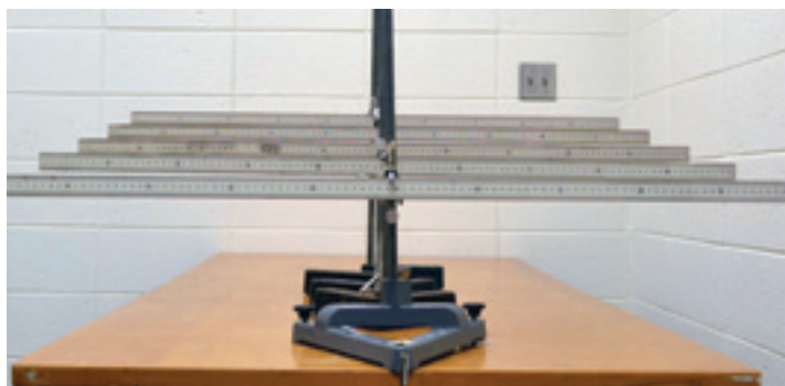
Meter stick array used to investigate motion in a different plane than the reference length. The middle meter stick was used as the “true” reference length.
