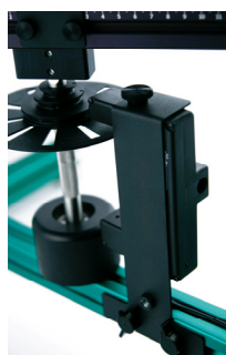
Dual-Range Force Sensor attached to frame, and with screw end of Swivel Assembly attached. Vertical adjustment screw on the right.
