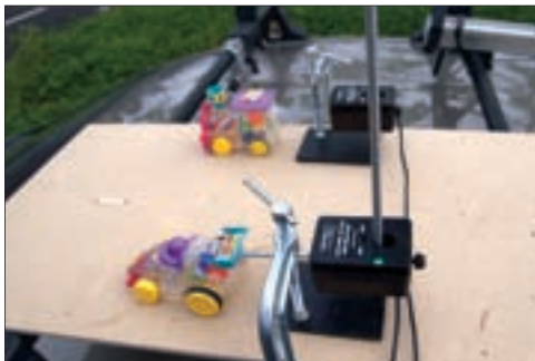
Two cars connected to Dual-Range Force Sensors to measure drag force
