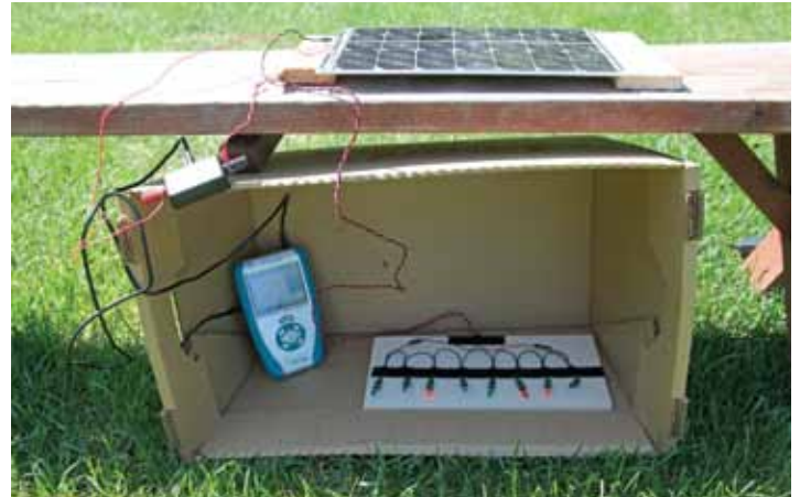
Solar panel, LabQuest with LEDs used as the load
