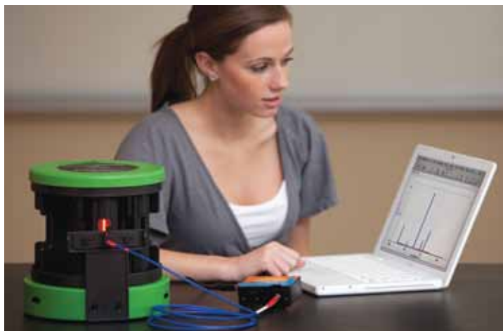
The Red Tide Emissions Spectrometer and Optical Fiber are used here with the Spectrum Tube Carousel Power Supply.
