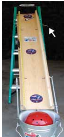
A weighted ball rolls down the ramp (left) crashing into a helmet containing the model head and accelerometer (above).
