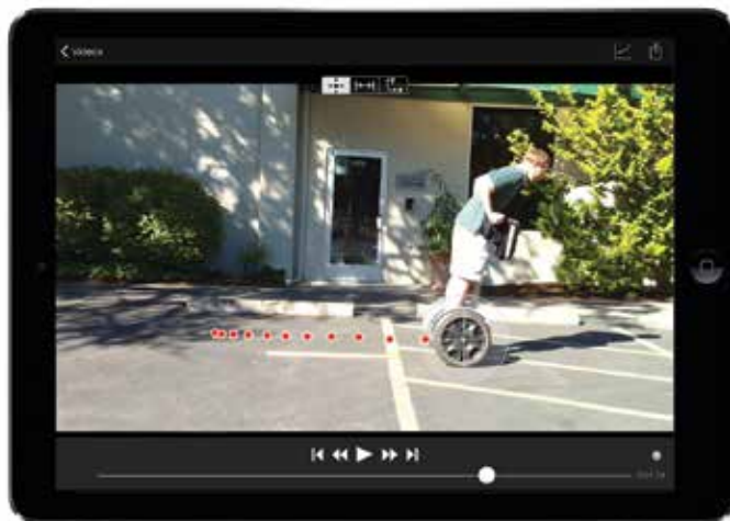
Video analysis of an accelerating Segway®
