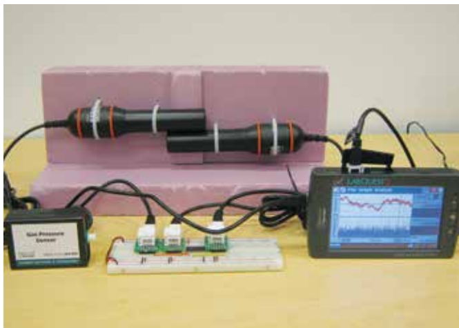
This is a muon telescope built from Vernier Radiation Monitors. Events that trigger both detectors are located along a line passing through both Geiger tubes.
