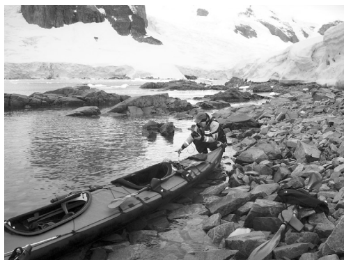
Heike Robinson, physics teacher and sea kayaker, measures the temperature of Antarctic waters with a LabPro, Palm, and Stainless Steel Temperature Probe.
