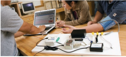
Student project: automated blood pressure monitor using SensorDAQ, Blood Pressure Sensor and the Digital Control Unit
